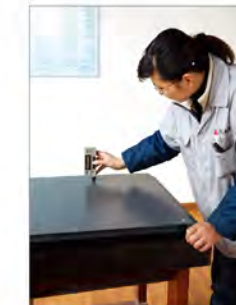
Coating Thickness Test 喷粉厚度测试
